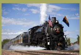
Steam locomotive No. 4960 was built in 1923. It was converted to use recycled waste vegetable oil for fuel, and reclaimed rain and snow melt are used in the boiler for steam.
